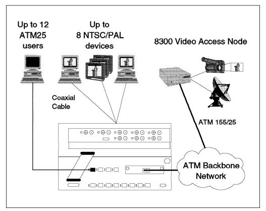
Figure 21. Video Distribution Module for Campus Video Distribution
